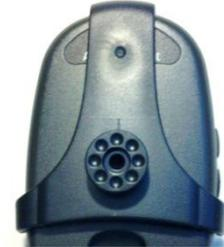
Once the belt clip is attached to the handset, Polycom does not recommend removing it for cleaning or other reasons.
