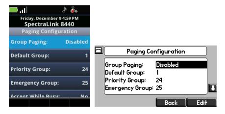
2 Make your changes to the paging configuration by highlighting a setting and pressing the **Edit** soft key.
