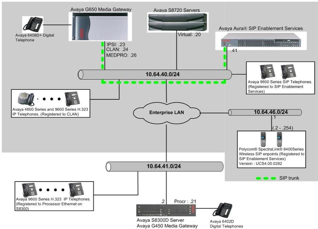
**Figure 1: Test Configuration of SpectraLink 8400 Series**
