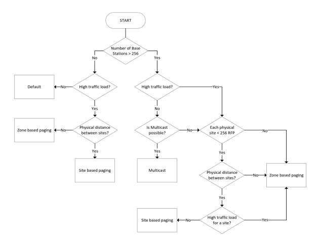
For more information about the different paging methods (default paging, multicast, site based paging and zone based paging) and the considerations that must be taken into account before configuring the IP-DECT base stations, see IP-DECT Server 200/400/6500 and Virtual IP-DECT Server One Installation and Configuration Guide. Please read the information carefully before continuing and ensure correct deployment of the base stations.
