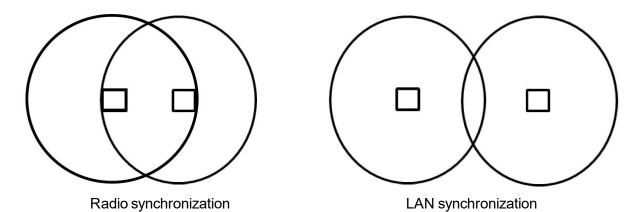
It should be noted, that depending on the deployment - LAN synchronization and radio synchronization can be combined in the same DECT installation. Even when a base station is configured to synchronize via LAN, it transmits the signal required for synchronization via radio. Therefore, base stations synchronizing via radio can retrieve their synchronization signal from a base station synchronizing via LAN. The other way around is not possible.
