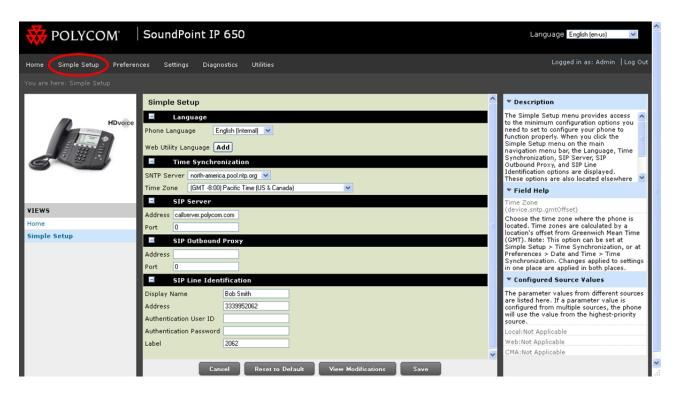
The Simple Setup menu is designed to help you quickly configure the most commonly used settings and features. These settings are also located in other menus throughout the Web Utility. Settings you apply in the Simple Setup menu are automatically set in the other areas.
