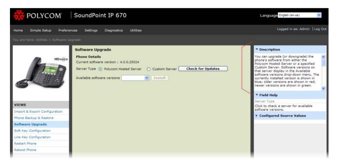
When you mouse over a setting on the user interface, the *Field Help* updates and provides you with the name of the parameter, some guidance about the parameter's function, and available settings. If a setting has been configured through another source, the setting will display under the *Configured Source Values* panel.
