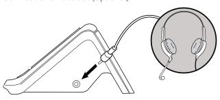
A wired headset may be used with the Speakerphone Dock. Plug it into the jack on the right side of the Speakerphone Dock and the audio will immediately route through it. If you are using a Bluetooth headset, audio will continue to flow through the Bluetooth headset when the handset is seated in the Speakerphone Dock.
