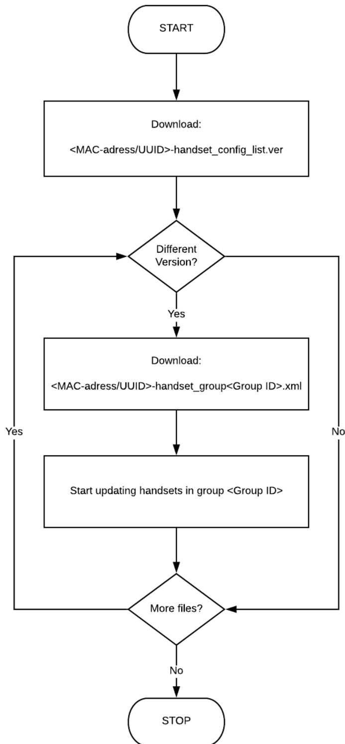
The [XML configuration file](#) is downloaded and imported into the Spectralink IP-DECT/Virtual IP-DECT Server and replaces the existing data. This guarantees that the data located on the provisioning server and on the Spectralink IP-DECT/Virtual IP-DECT Server are identical.
