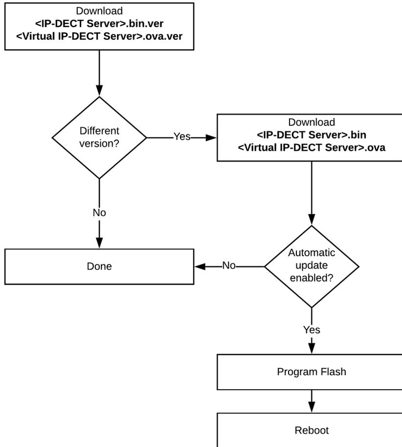
The firmware version specified in the ".ver" file is compared with the firmware version that is currently executed. To avoid problems with different firmware versions being executed and program flash, the Spectralink IP-DECT/DECT/Virtual IP-DECT Server is rebooted immediately after the firmware is updated.
