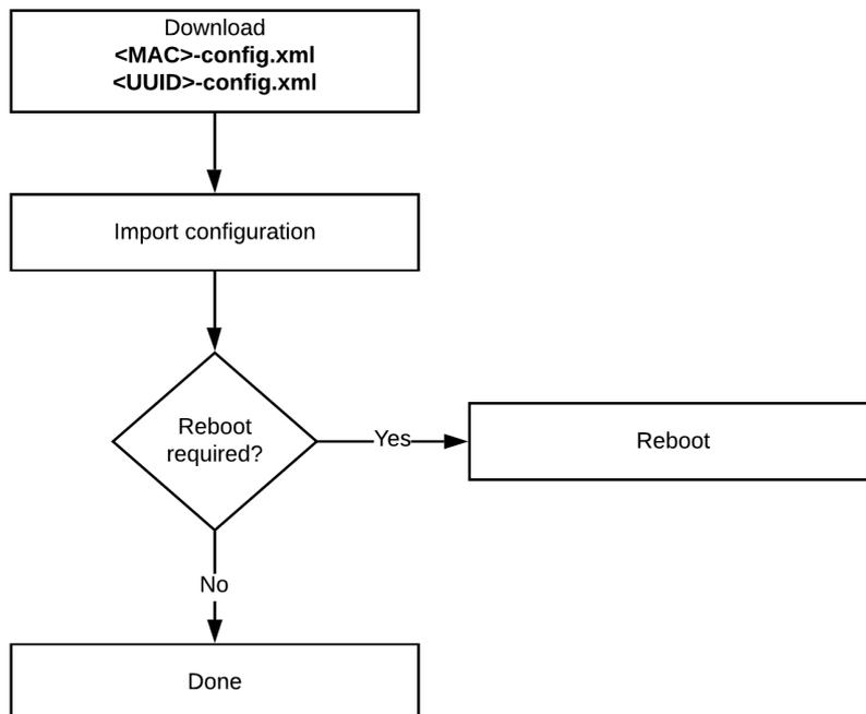
The [XML configuration file](#) is downloaded and imported into the Spectralink IP-DECT/DECT/Virtual IP-DECT Server configuration by replacing the existing data. This guarantees that the data located on the provisioning server and on the Spectralink IP-DECT/DECT/Virtual IP-DECT Server are identical.
