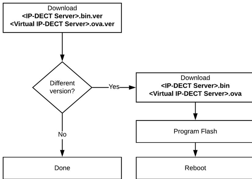
Example of provisioning of firmware for base stations, media resources and handsets with Enhanced Provisioning License installed:
