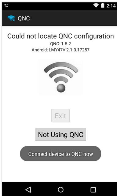
This error is usually caused when the configuration has not been saved. Re-configure QNC settings and click the Save button on each screen.
