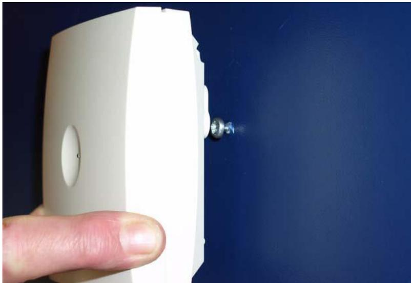
**Figure 13 – IP-DECT Server 400 / Base station Wall mounting**
