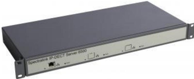
Mount the two wings with the included screws as shown in above picture. If you are mounting it on a wall, twist the brackets 90° degrees. Then mount the server in a 19” Rack cabinet or upwards on a wall.
