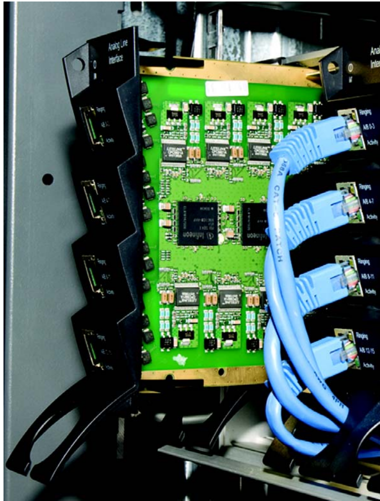
Figure 8 Installing Interface Cards
