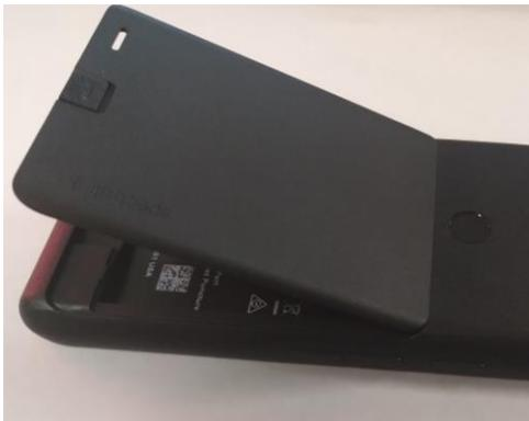
1. Finally, gently withdraw the battery tabs from the battery compartment cavities and lift the battery out of the battery compartment. Make sure that no part of the battery drags across the Versity battery contacts.
