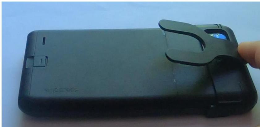
Figure 12 - Insert or Remove a battery with the clip lever activated trying not to impact the Versity battery contacts.
