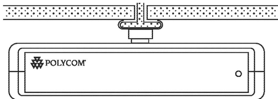
4. When properly attached the Base Station should sit almost flush against the ceiling and be tightly attached to the clip and T-bar grid work.
