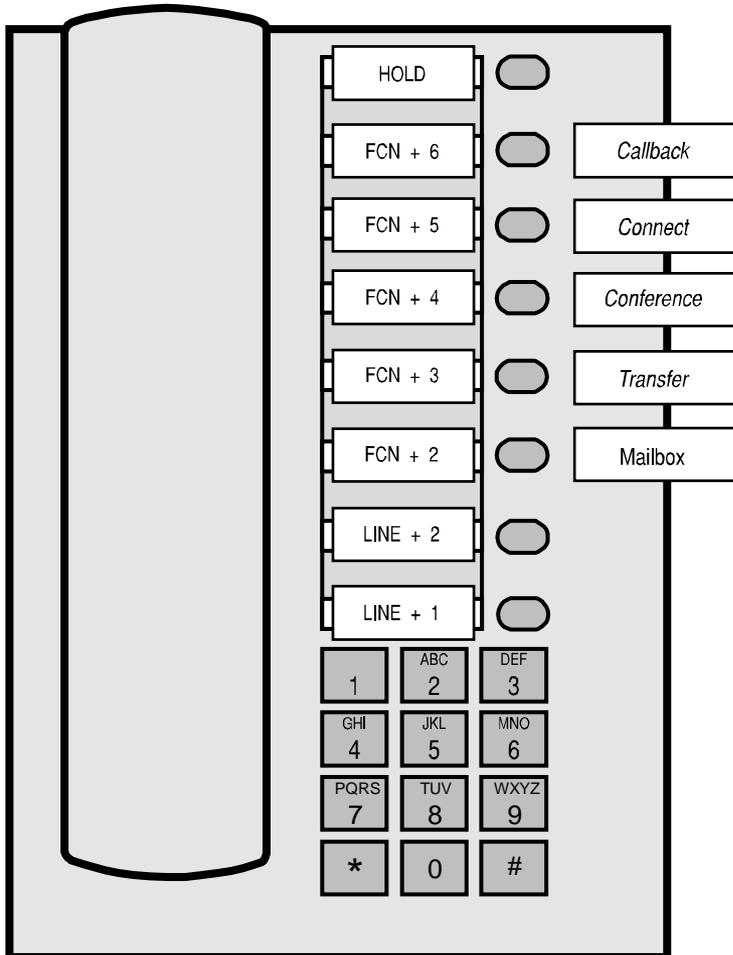
The **FCN** and **LINE** labels represent the key sequence on the handset mapped to the corresponding key on the optiset E. The feature labels to the right of the keys represent one possible mapping scheme, but any feature may be programmed to keys that do not have setup restrictions described in the Feature Programming Requirements section.
