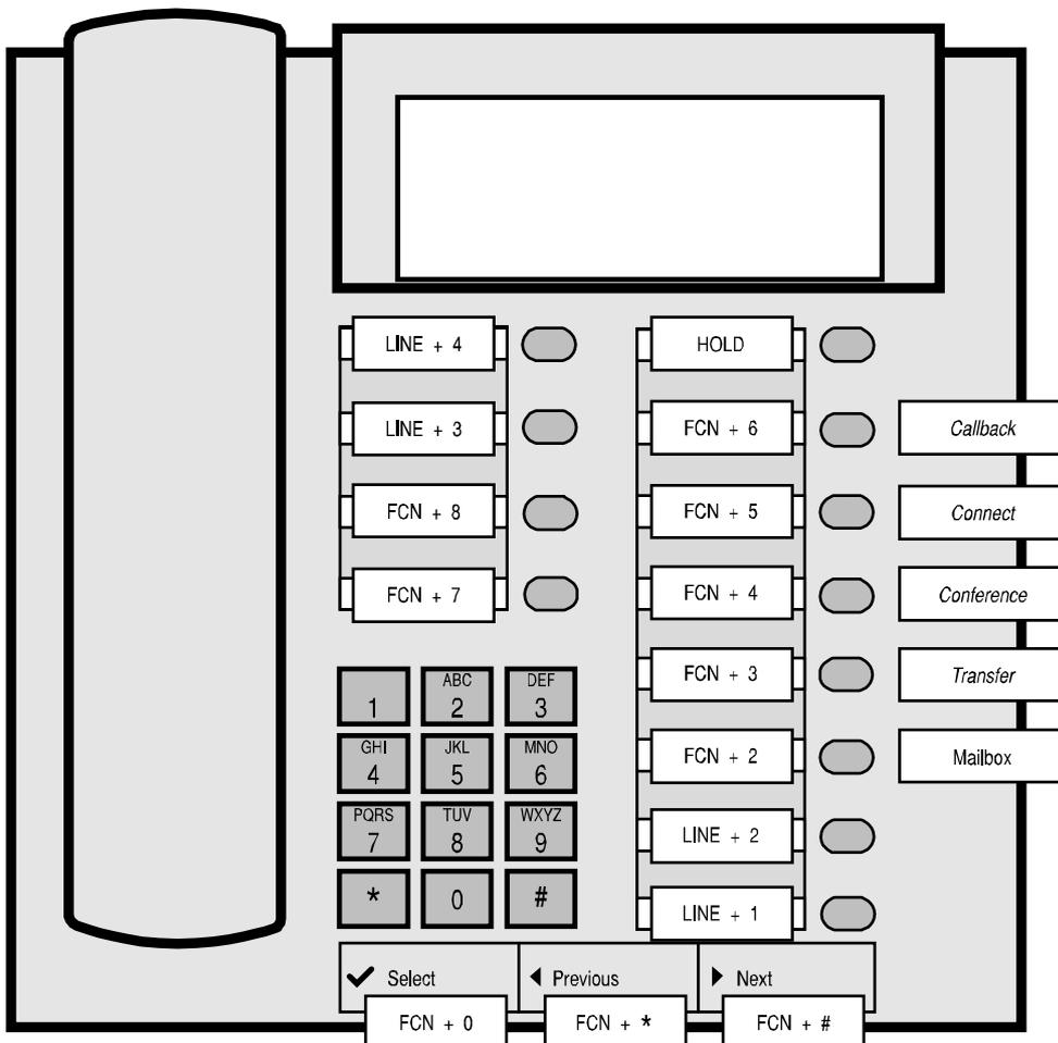
The **FCN** and **LINE** labels represent the key sequence on the handset mapped to the corresponding key on the optiset E. The feature labels to the right of the keys represent one possible mapping scheme, but any feature may be programmed to keys that do not have setup restrictions described in the Feature Programming Requirements section.
