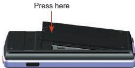
Gently press the top of the Battery Pack until it snaps into place. The Battery Pack should snap into position with minimal pressure.
