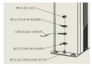
No more than 15 units may be grounded though one connection to the protective earth ground. Systems with more than 15 units must be separated into groups of 15 or less with each group having their own independent protective earth ground connectors.
